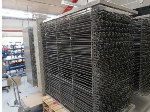
Insulated resistance heater bank for air heating (Source: SAN Electro Heat)
