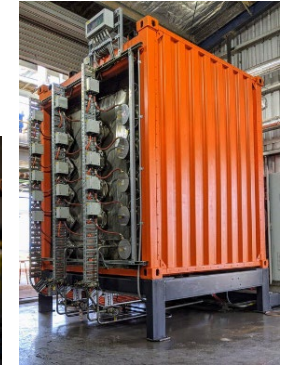
Graphite Energy, storage in graphite, radiative electric charging, water/steam discharging
